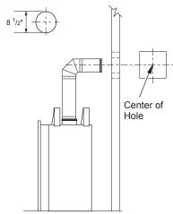
Figure 9 - Vent Opening Requirements
